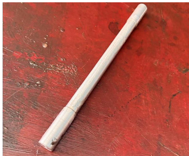
Fig.7. Aluminium shaft after machining
