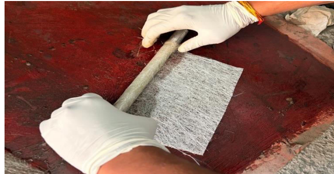
Fig.8. Reinforcement of Glass fibre and sisal fibre layers
