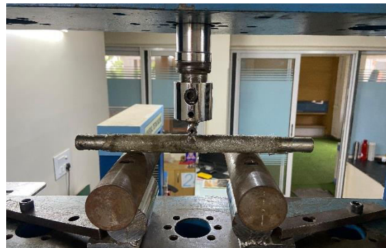
Fig.10. Specimen under Flexural test using UTM
